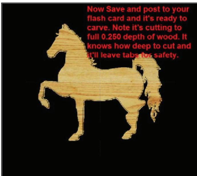
14. Now you have the finished project of an image cutout. Cut Path operation has automatically built in “tabs” so the cutout part will not get caught by the bit and harmed. The project is ready to be uploaded onto your CarveWright/CompuCarve Flash Card, and then put into the machine and carved.
